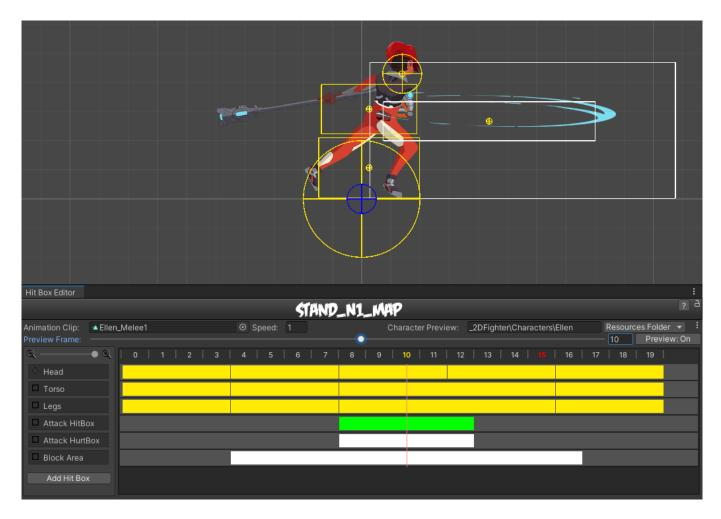
To add a new hit box click on **Add Hit Box**. Right click on it to display all the options for the hitbox such as shape, collision type and hit type.
